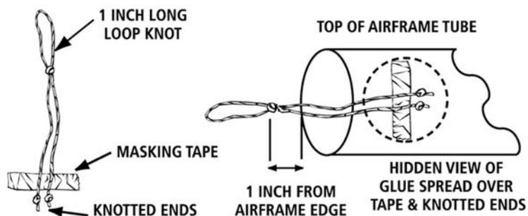
3. Carefully place the two knotted loose ends of the Shock Cord Mount, with tape attached, inside the top of airframe tube so that the 1" long loop knot is protruding out about 1" from the airframe tube's edge. Using a small piece of wooden dowel, press the masking tape down firmly around the inside of the airframe tubing. The masking tape will keep the Shock Cord Mount in place while gluing.
